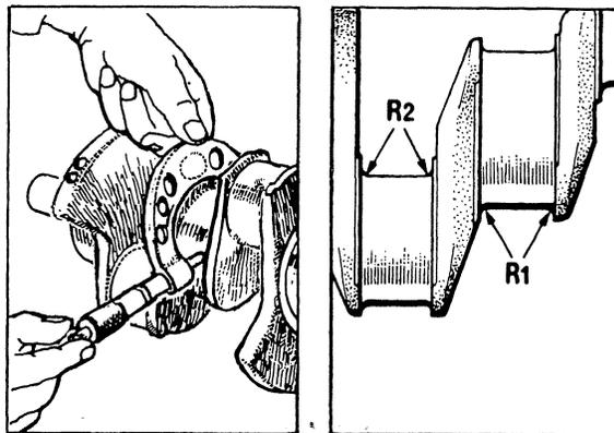
b. Using a micrometer, measure each crankpin (take a total of four readings) to determine the wear, out-of-round and taper. If any of the limits is exceeded, repair by grinding to the next undersize or replace the crankshaft.
