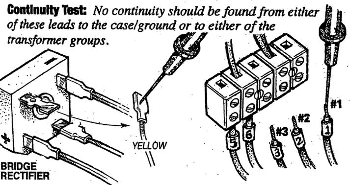
**Continuity Test:** No continuity should be found from either of these leads to the case/ground or to either of the transformer groups.
