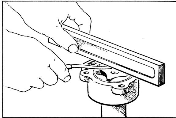
Checking rotor-to cover clearance
