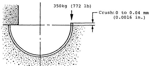
Connecting rod bearing crush
