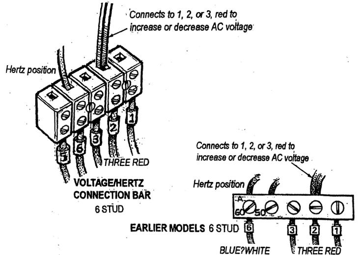
connections are generally used to increase excitation when at full amperage load the AC output of the generator falls below acceptable levels 108 volts – 60 hertz or 210 volts – 50 hertz. Note: Hertz/Speed drop is not the issue. No-load voltage may need to be adjusted when these connections are moved.
