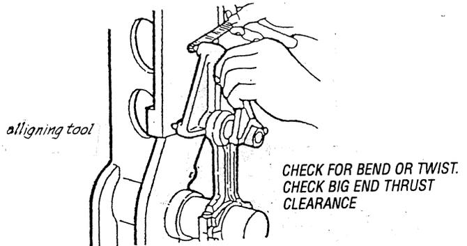
Checking connecting rod for bend
