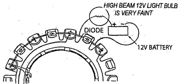
Reverse the leads across the diode. The diode should block voltage passing through it, and the headlight should not glow, or it may glow faintly.
