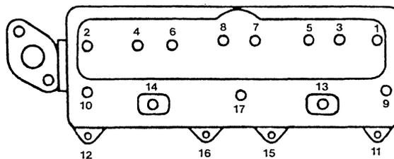
Cylinder Head Bolt Tightening Sequence
