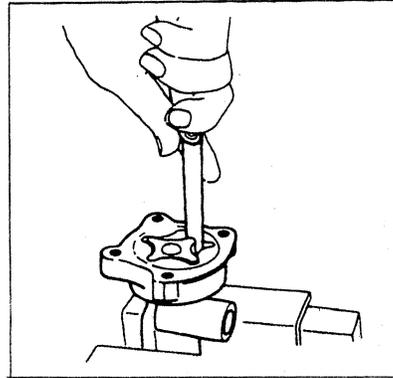
Checking rotor-to-rotor clearance
