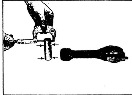
Use a micrometer to measure piston pin bushing and piston pin
