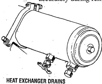
HEAT EXCHANGER DRAINS
