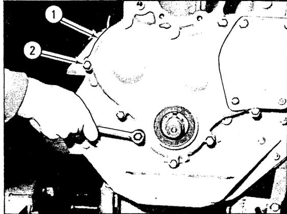
20. Install front crankshaft pulley. Take care not to damage front crankshaft seal when slipping pulley onto crankshaft and through the front seal.
