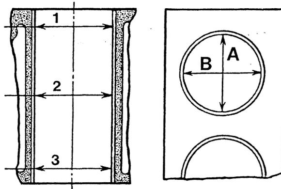
Positions for checking sleeve bore diameter
