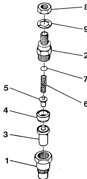
Injection Nozzle Assembly - Disassembled View
