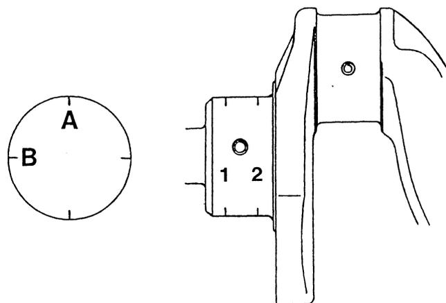
Positions for measuring journal with a micrometer
