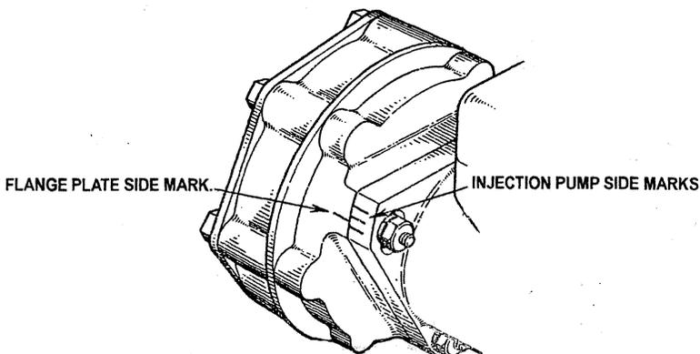
Scribe mating marks on the pump body and the timing gear case before removing.
