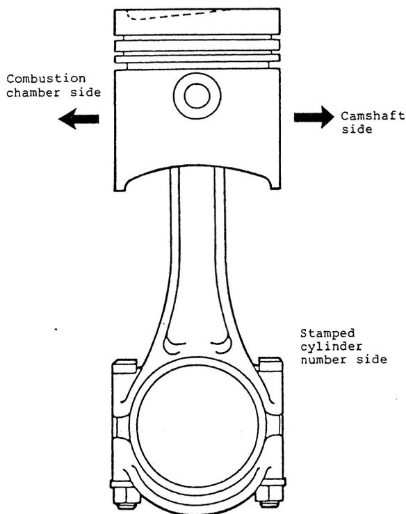
Piston and connecting rod assembly
