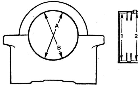
Positions for measuring main bearing
