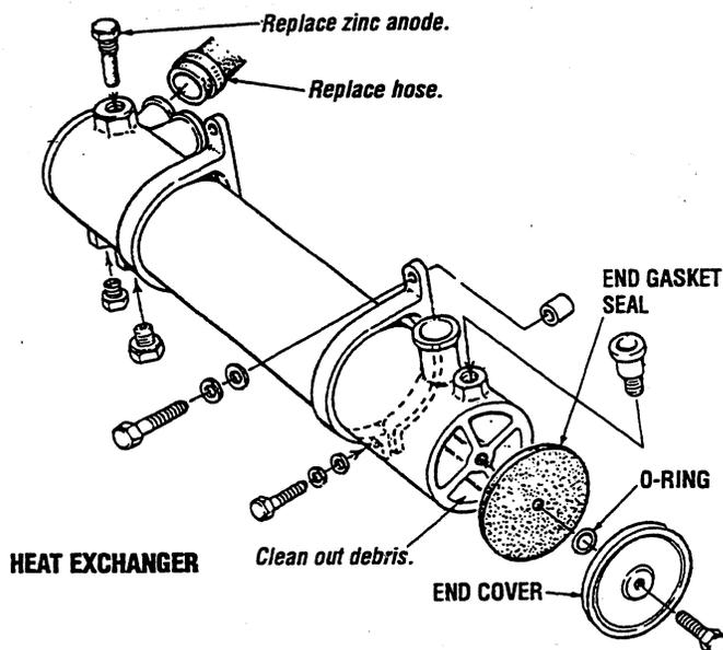
**NOTE:** *All of the above can be accomplished by sending the heat exchanger to a radiator shop. They will also service transmission and engine oil coolers.*
