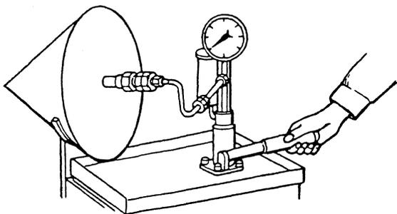
Checking injection pressure on nozzle tester
