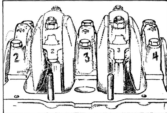
10. Remove the main bearing caps by loosening and removing the attaching bolts.
