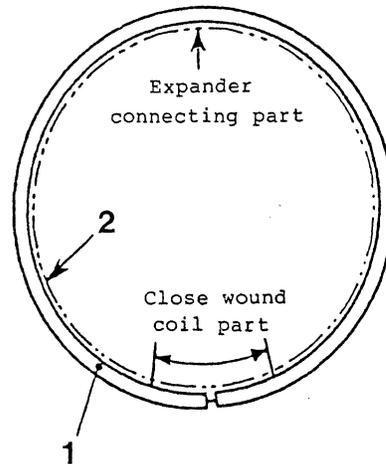
Oil control ring and expander installed
