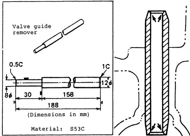
Valve guide removal tool    Wear on valve guide
