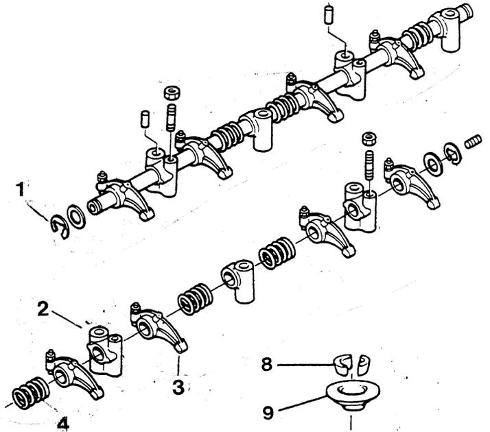
15. Disassemble the cylinder head as follows:
