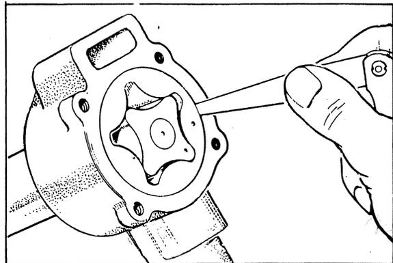
Checking rotor-to-body clearance
