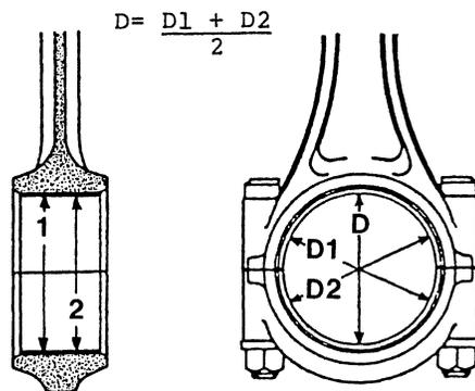
Positions for measuring connecting rod bearing with a micrometer
