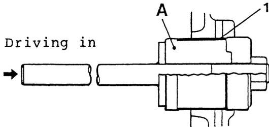
Driving in camshaft bushing
