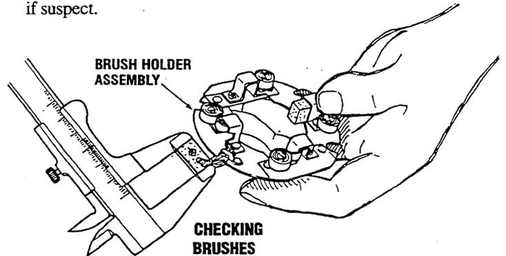
3. Check for insulation between the positive brush holder and holder base. If poorly insulated, replace the holder assembly. Also check the brush holders for proper staking.
