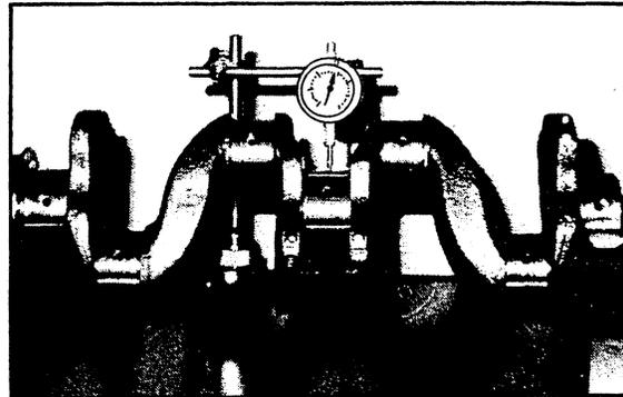
Checking crankshaft for runout
