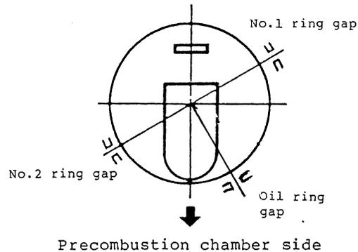
(NOTE: Piston/rod assembly is installed from crankshaft side of engine block.)
