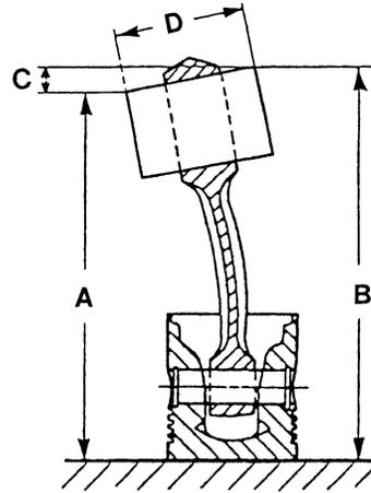
Checking connecting rod on surface plate
