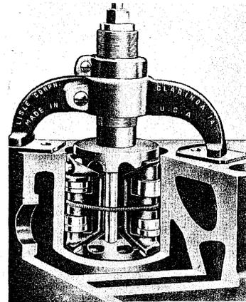
Removing ridge with ridge reamer
