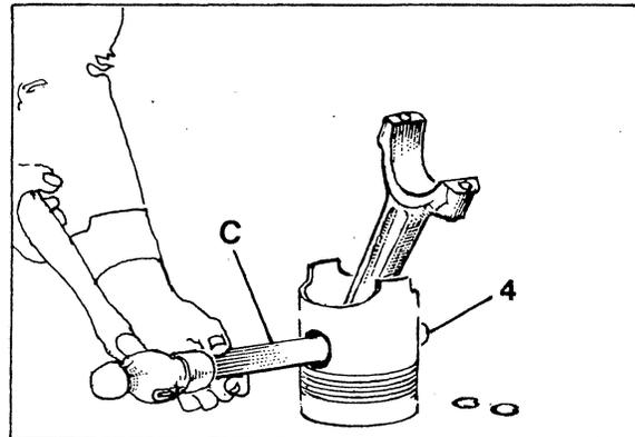
(NOTE: Heating the piston by resting the piston crown down on an electric hot plate will allow for easier removal of the piston pin.)
